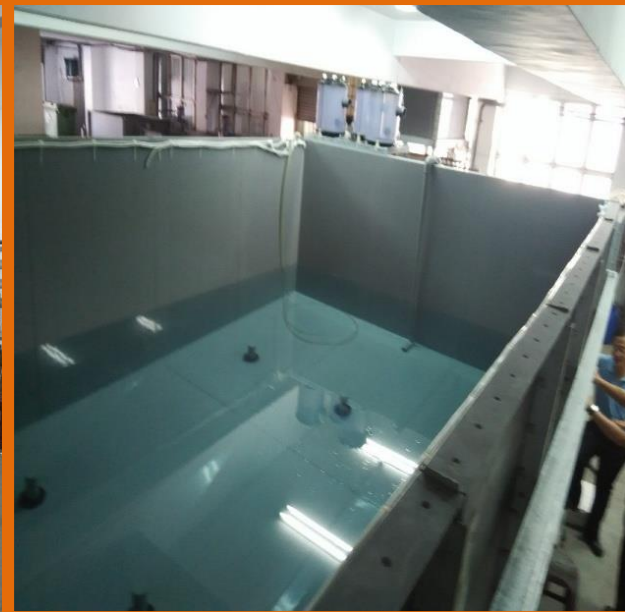
操作容水量：31,000L Aquaculture Panel Type Water Tank Inside Operation Water Capacity：31,000 L
